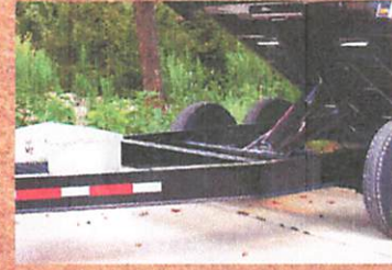
8" I Beam Frame
